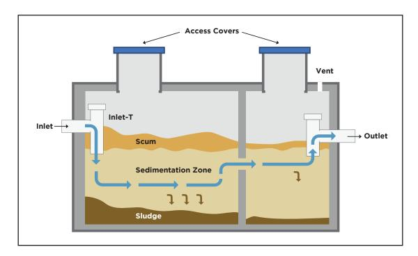
The speed at which solids accumulate in the septic tank is impacted by the number of people using the septic system, the type of water use, and many other household characteristics. The only way to really know when your septic tank needs to be pumped is to measure how many solids are in the tank. A maintainer will do this as part of their routine inspection.
