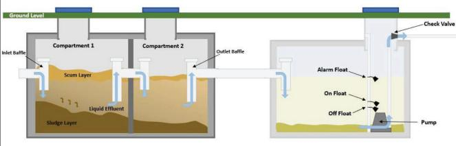
This diagram shows the contents of a pressure distribution septic tank and pump tank.
