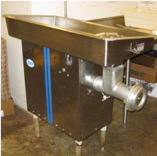
New meat grinder with fixed guard (tray)
