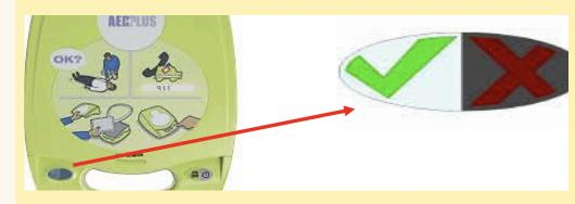
If something needs attention, the AED will indicate it by a beep, a flashing red light, a red "X", etc. A chirping sound typically means maintenance is required.
