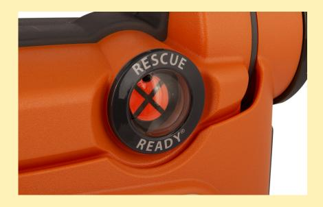
If the AED shows no status indicator at all, ensure the AED is turned on and check the AED immediately for the cause, including the possibility of a dead battery. If an AED is inoperable, remove it from service.
