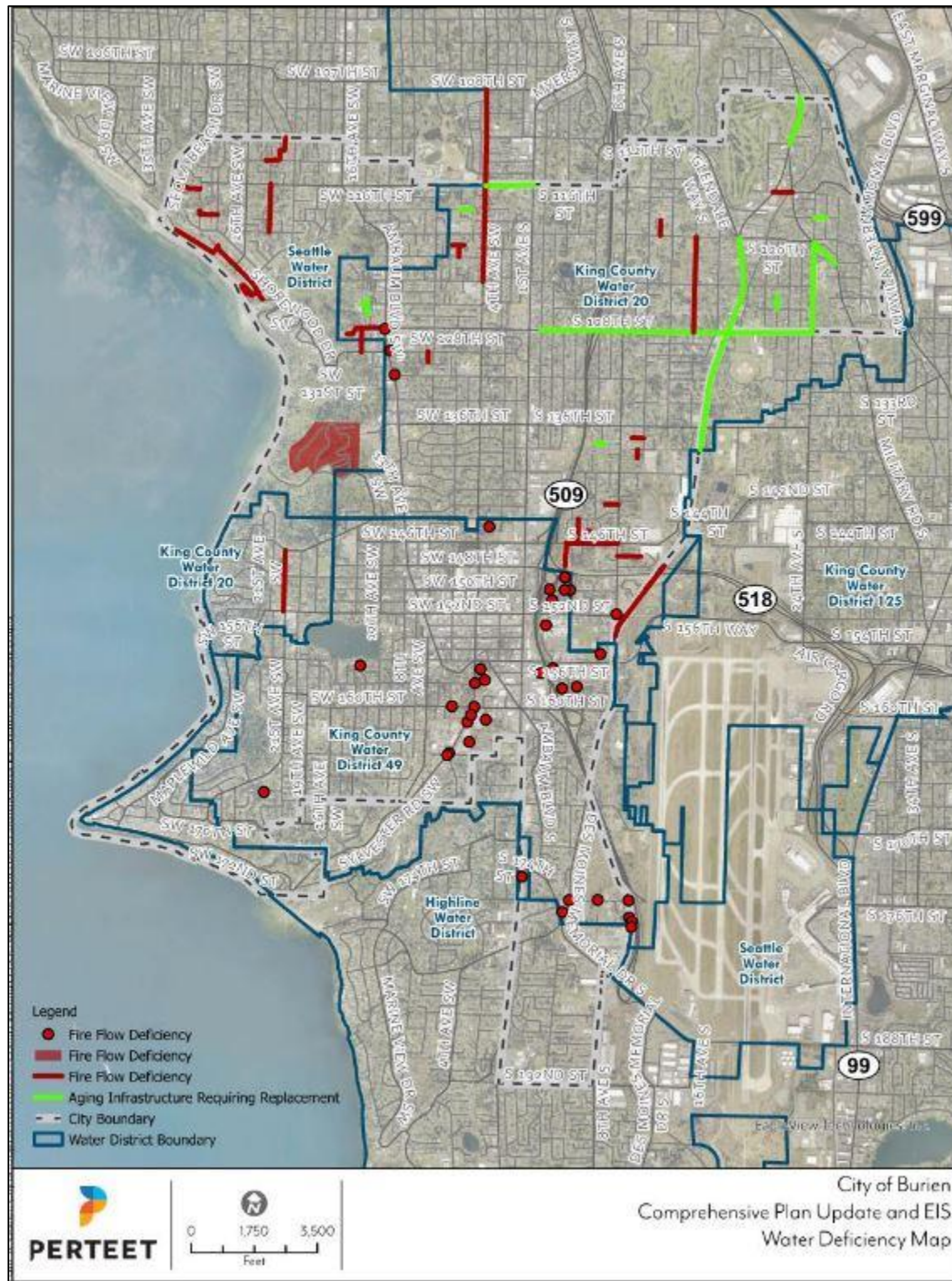
Fig. 9: Water System Deficiencies in Burien
