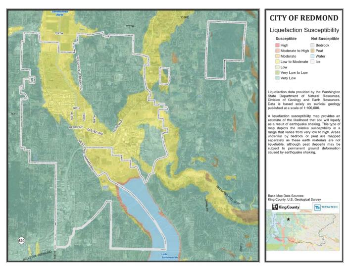
Figure 2: Liquefaction Susceptibility.
