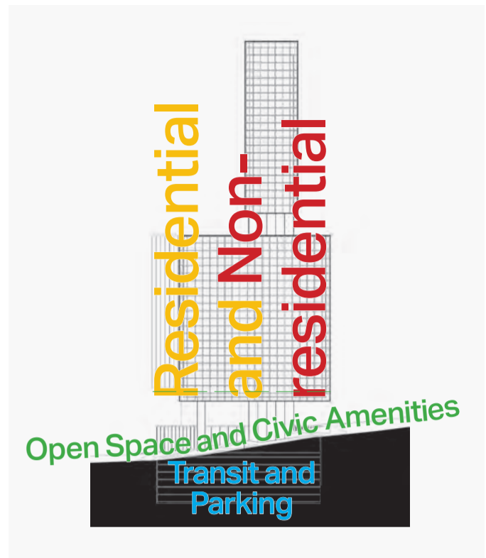
Strategic diagram illustrating the vertical layering of functions on potential redevelopment sites.
