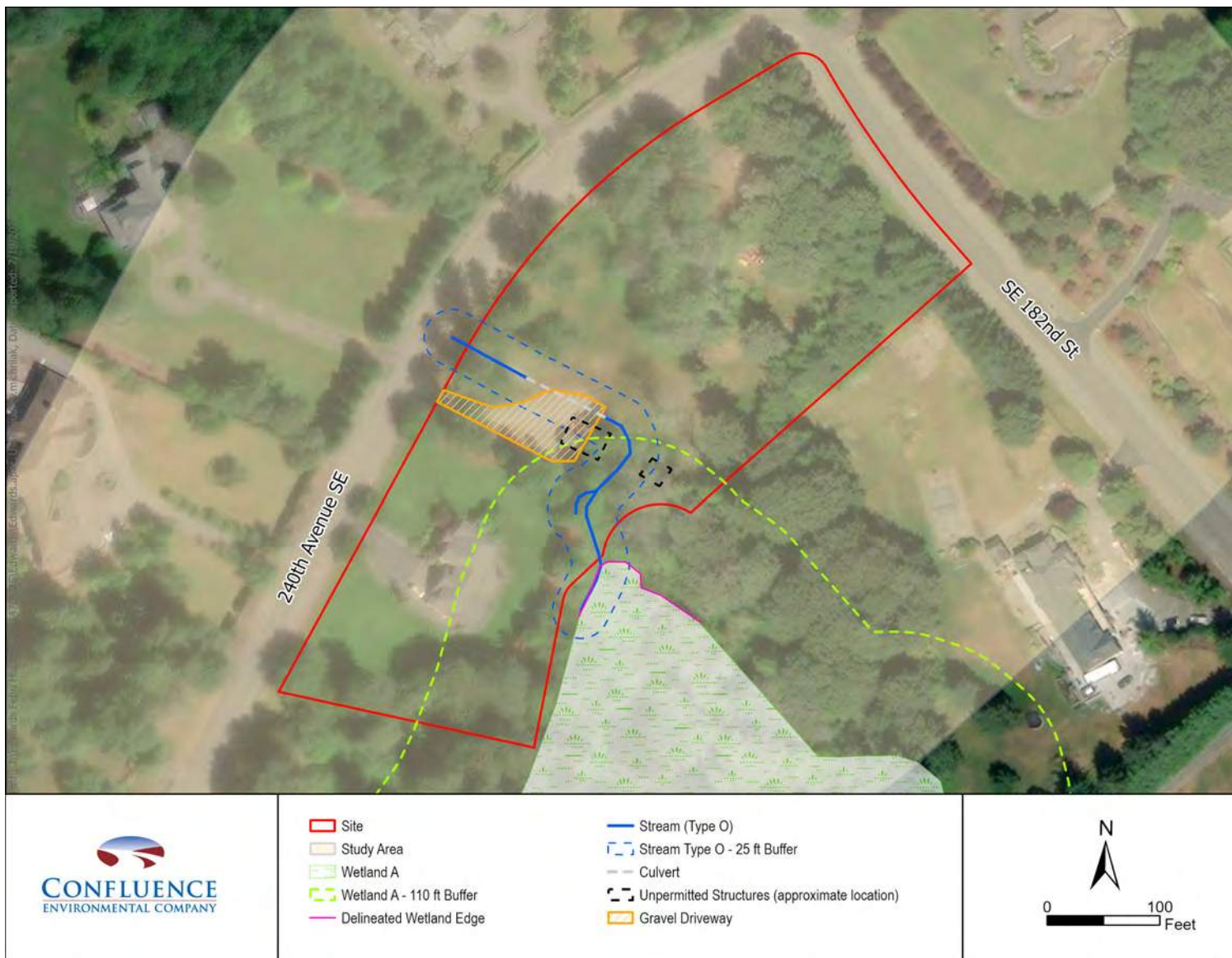
Figure 3. Wetland A and stream buffer
