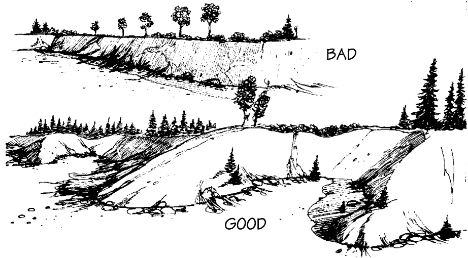
Figure 4.3. A key element in restoring topography is creating natural-looking slopes that blend with the surrounding landforms. Rectilinear slopes (top) are inappropriate for reclamation in unconsolidated materials. Slopes should be curved in plan and section and irregular in profile (bottom). (Redrawn from Green and others, 1992.)
