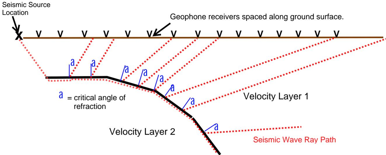
The figure shows the effect of a steeply sloping velocity layer. Seismic waves are refracted from the Velocity Layer 2 surface at the critical angle ( $a$ ). For steeply sloping interfaces the ray path will not be refracted back to the geophones at the ground surface. The length of the geophone array will also be a factor in detecting the refracted energy.
