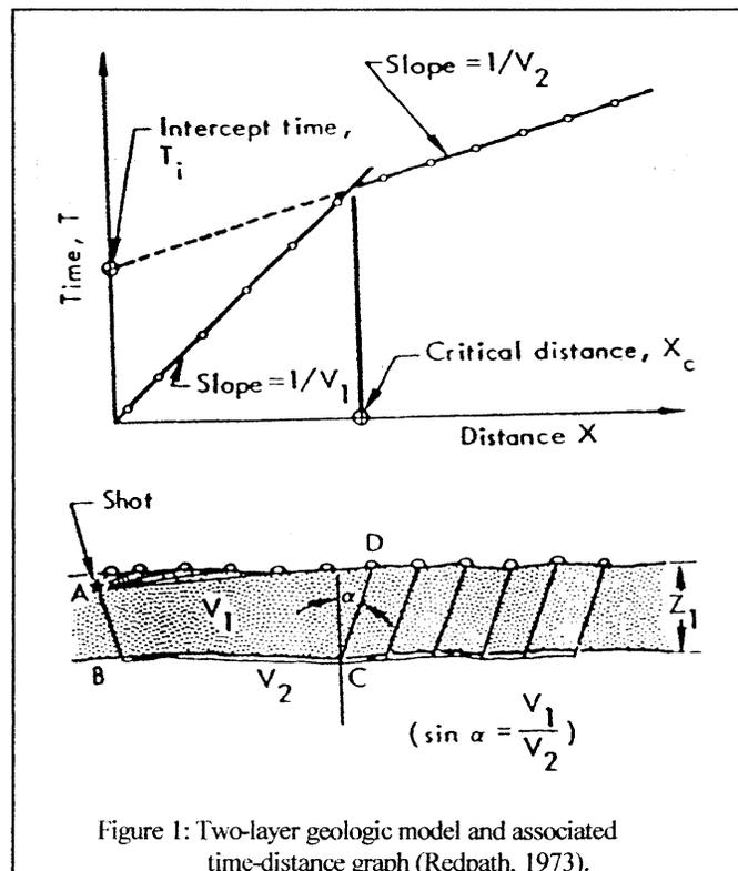
Figure 1: Two-layer geologic model and associated time-distance graph (Redpath, 1973).
