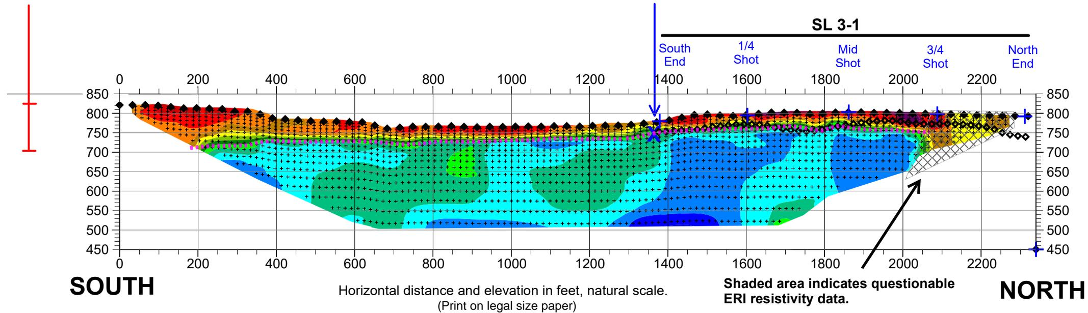
**Model Resistivity Contour Values (ohm-meters)**
