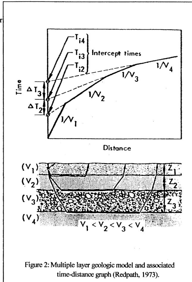
Figure 2: Multiple layer geologic model and associated time-distance graph (Redpath, 1973).
