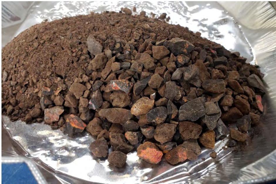
Photograph 16. Example of samples before being sieved through a 3/8-inch sieve to obtain appropriate size for TCLP and SPLP analysis.
