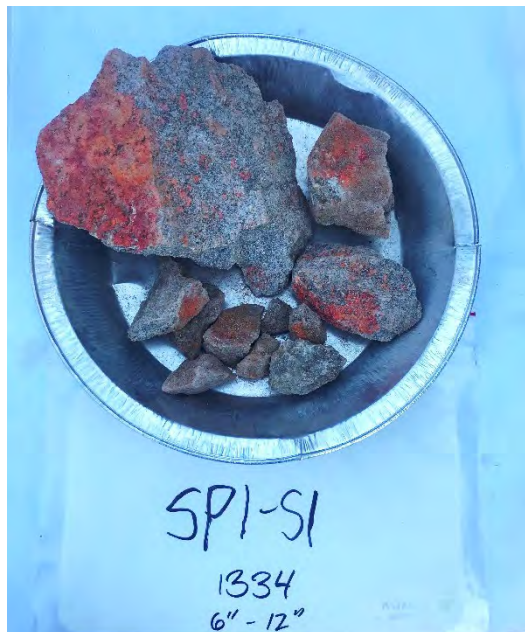
Photograph 14. Samples taken on August 30, 2022, were collected in zip-block bags as shown. Some of these samples were too large to be analyzed by the laboratory (similar to photo above) so Aspect crushed and sieved the rocks to an acceptable size.
