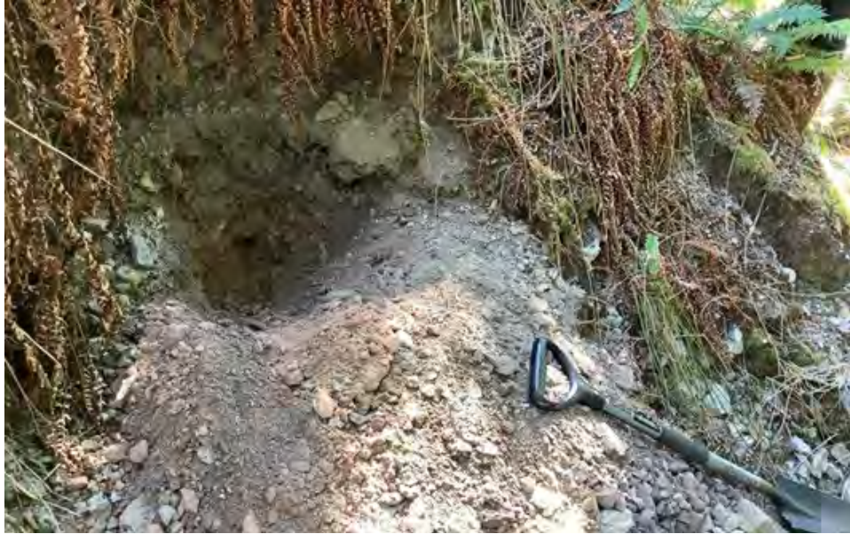
Photograph 7. Stockpile 1 exploration. Several samples were taken from different locations around this stockpile. This stockpile was uphill from the former hearth furnace and Stockpile 4. The ore in Stockpile 1 appears to be “raw” and unprocessed (i.e., the ore does not appear to have gone through the furnace and vibrant crystals of sulfide minerals were visible on many of the pieces of ore observed).
