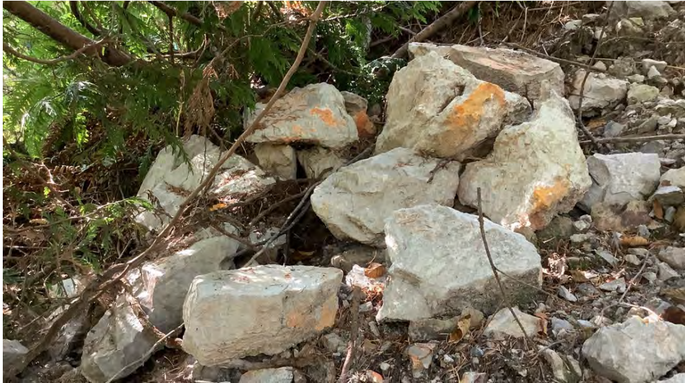
Photograph 9. Example of typical waste rock observed at Stockpile 1. Some of the ore had vibrant red, orange, or yellow crystals, characteristic of various sulfide minerals such as realgar, cinnabar, and orpiment.
