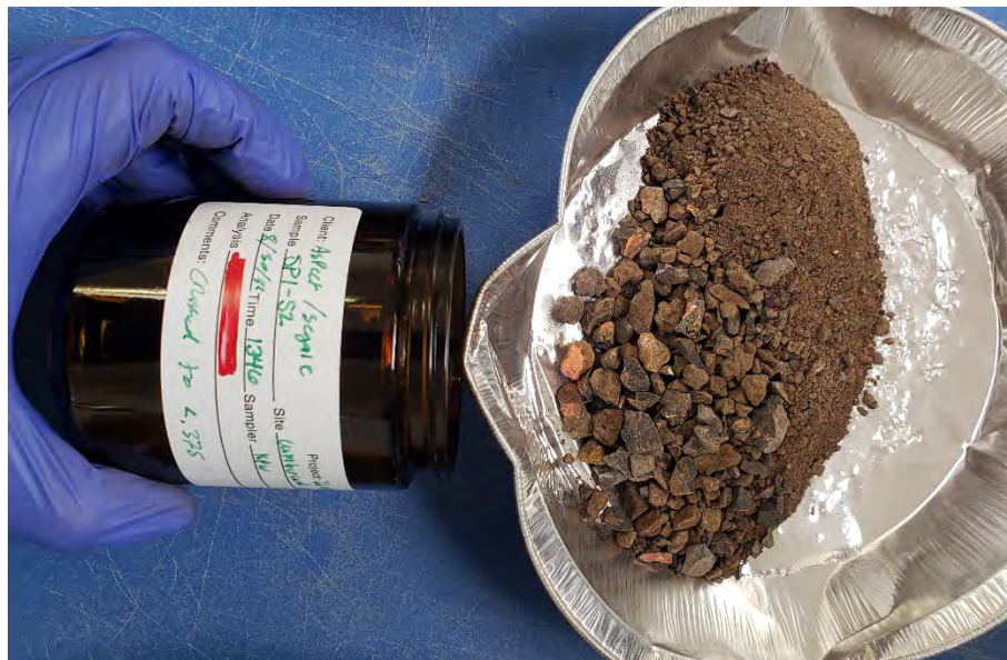
Photograph 18. Example of sample after completing crushing and sieving process to obtain appropriate size.
