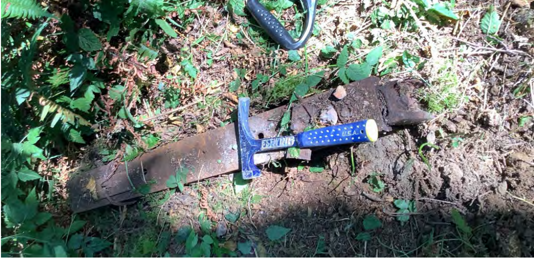
Photograph 13. Metal bar protruding from Stockpile 4 (geologic hammer for scale).
