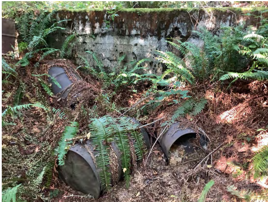
Photograph 6. At least four 55-gallon drums containing solid granular material were observed near the southeast corner of the former hearth furnace. The drums were in poor condition, were not sealed with lids, and were overgrown with native vegetation.
