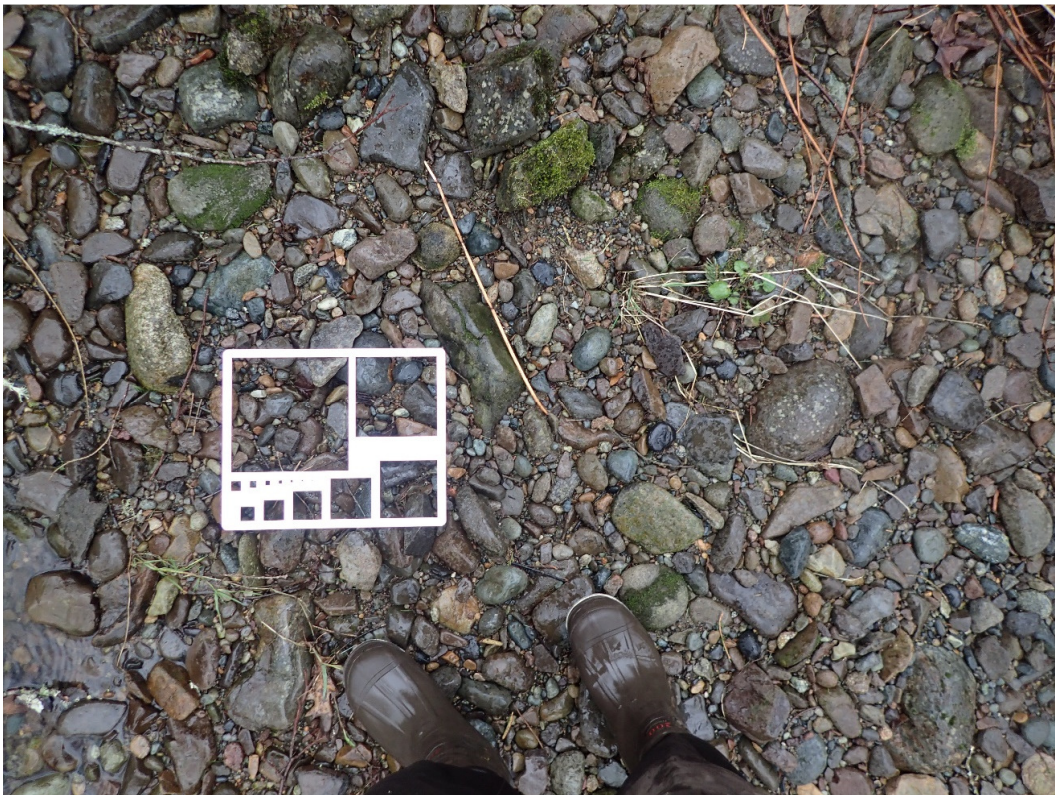
Gravelometer on LB point bar at location of pebble count. (Photo N)
