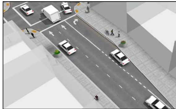
Example of a right turn pocket.
