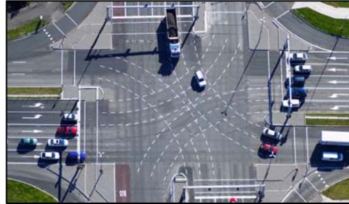
A channelized intersection example.
