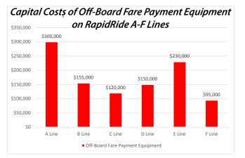
Off-board fare payment equipment helps achieve faster bus travel times by decreasing the dwell time at stations. Buses are able to load more quickly because riders have paid prior to the bus arriving and can also enter through any door. A study of the impacts of installing
