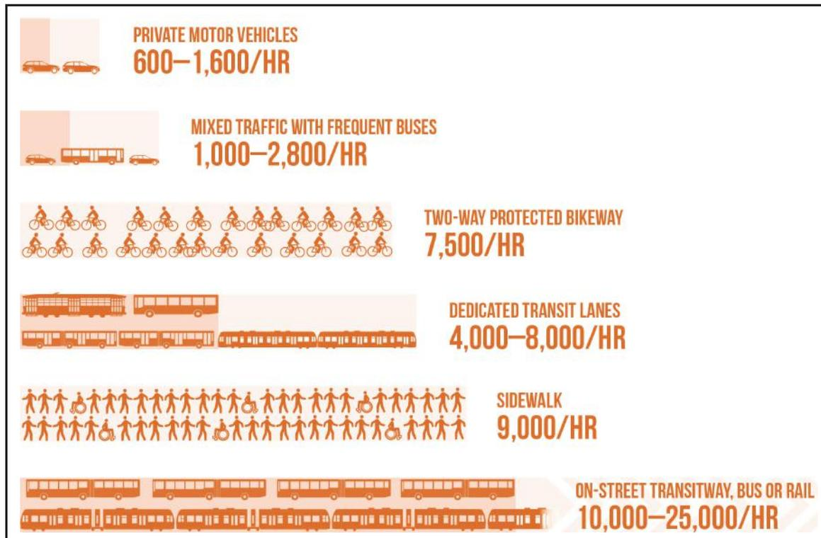
The capacity of a single general-purpose traffic lane by mode at peak conditions with normal operations.
