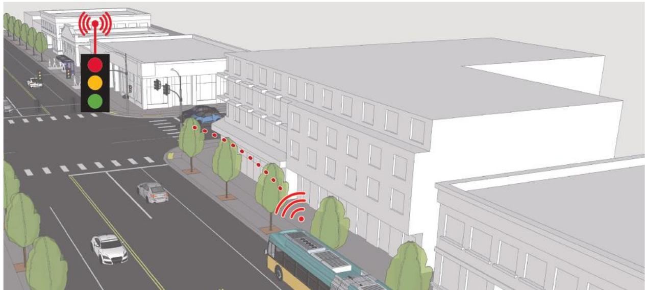
late and request different levels of priority in response. All new TSP installations will use King County's next-generation TSP system using center-to-center (C2C) connections and existing city-owned communications networks.
