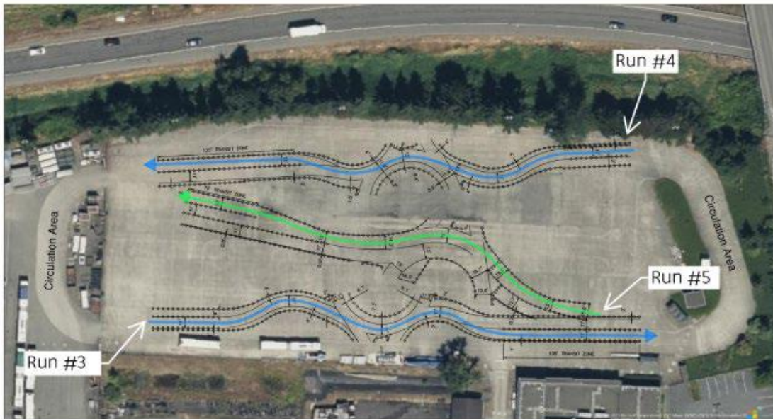
Figure 8: Layout for coach testing of the I-405/North 85 th Interchange roundabout design.
