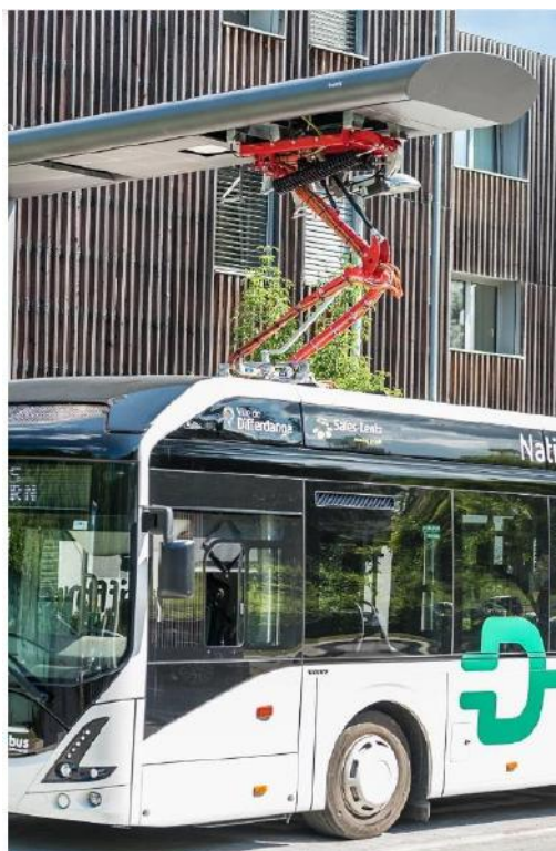
Figure 5. Overhead charger with an inverted pantograph (moving parts on charger, not on the bus)
