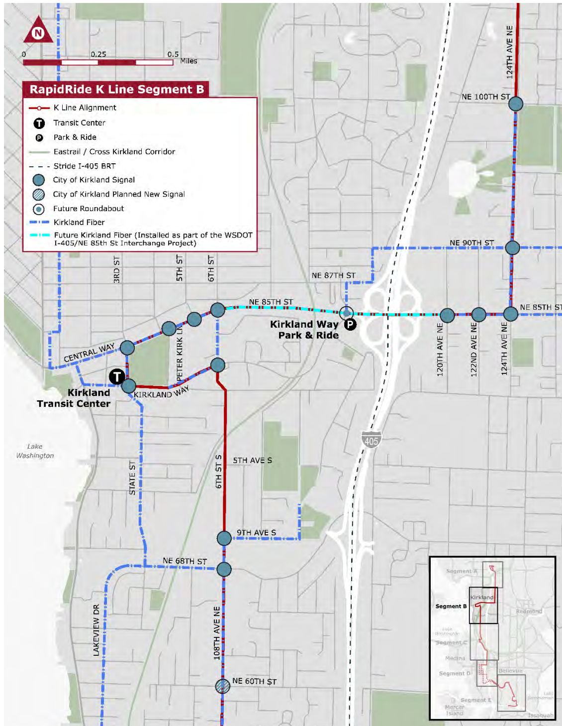
Figure 3-2. Segment B Existing Fiber & Existing Signals
