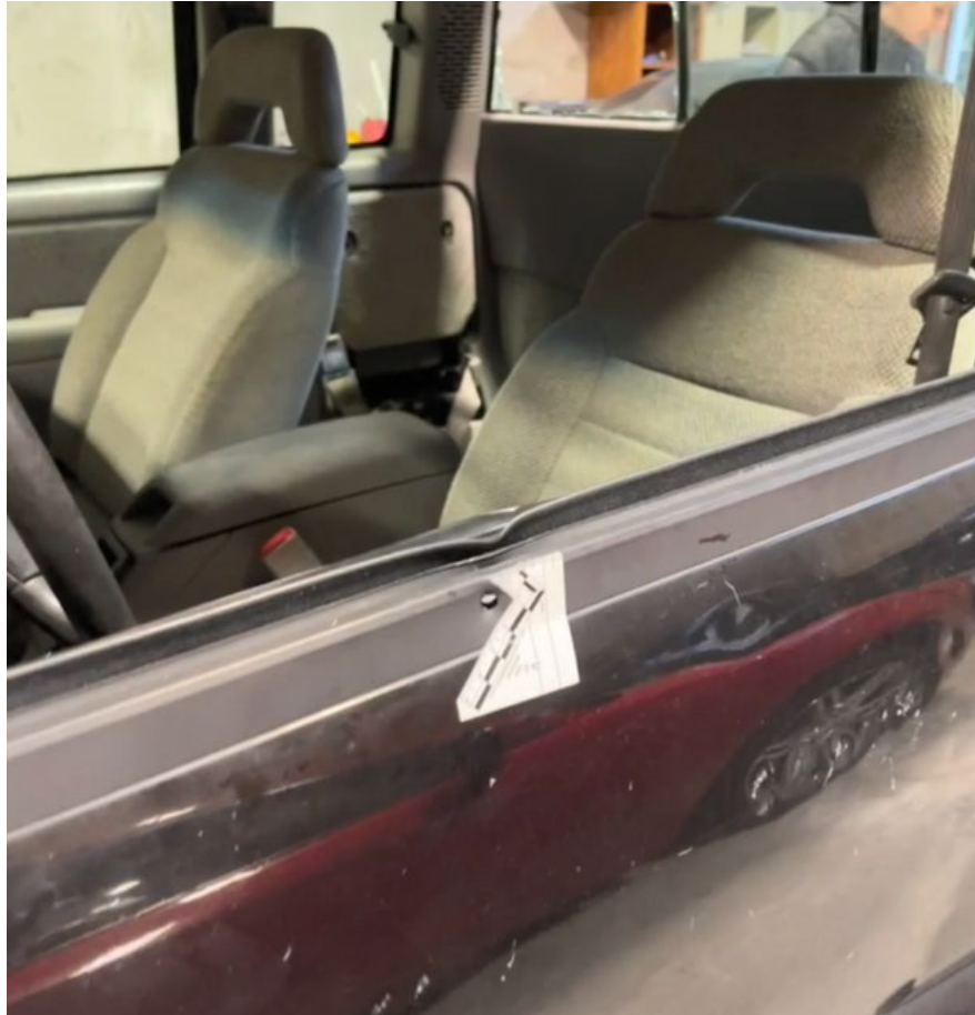
Caption: Angle of bullet defect E entering and exiting the driver side door.
