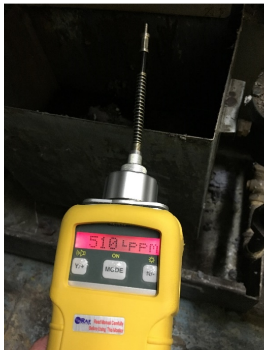
Figure 1. Using a PID to detect PERC The reading of 510 ppm was taken at the still bottom (sludge) waste container next to the still door
