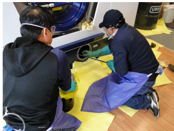
Figure 5. Clean out PERC tanks with rod and absorbent pad. Photo by Stephen G. Whittaker, King County
